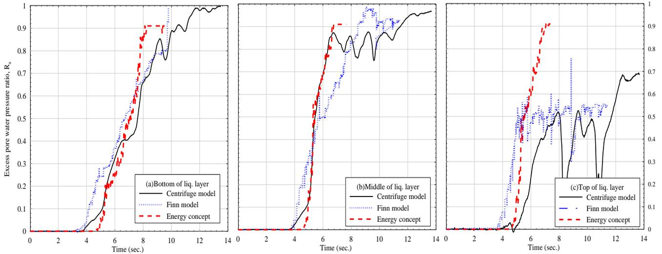
Figure 4. Comparison between the measured and estimated pore water pressure at (a) bottom (b) middle, and (c) top of the loose Ottawa sand layer.
