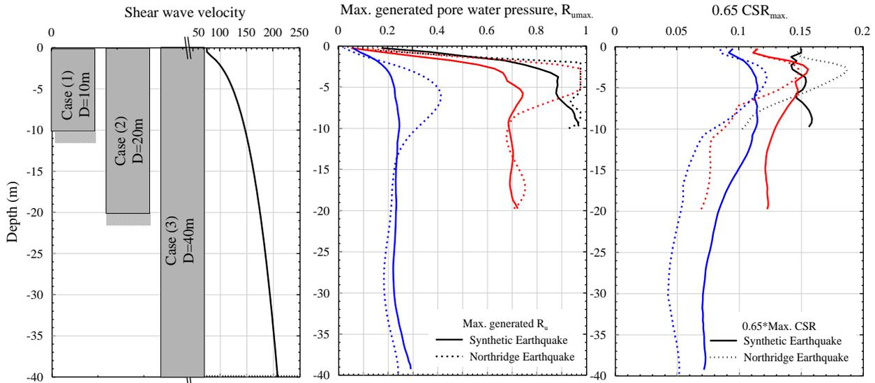
Figure 6. (a) Shear wave velocity and (b) maximum average cyclic stress ratio and generated pore water pressure ratio,  $R_u$ , calculated by 1D linear analysis along depth in the uniform soil deposit by 2 earthquake motions.
