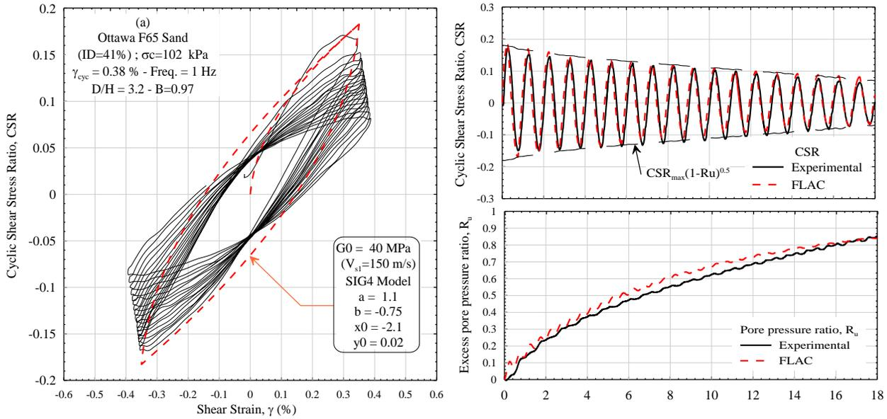
Figure 2. Typical results of TxSS test and numerical model in terms of (a) Hysteresis loops ( $CSR-\gamma_{cyc}$ ), (b) CSR time history, (c)  $R_u$  time history.
