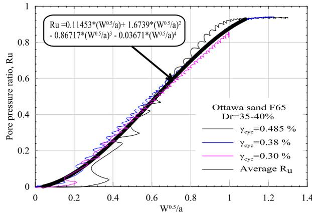
Figure 1:  $R_u$ - $W_s$  relation after strain-controlled tests
